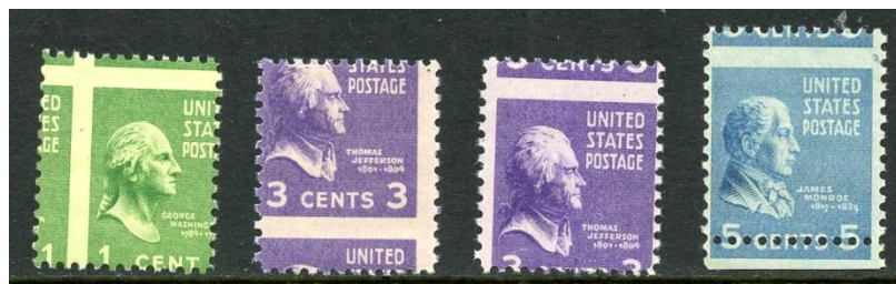
Figure 8. Improper perforations due to incorrect alignment of the rotary perforators.
