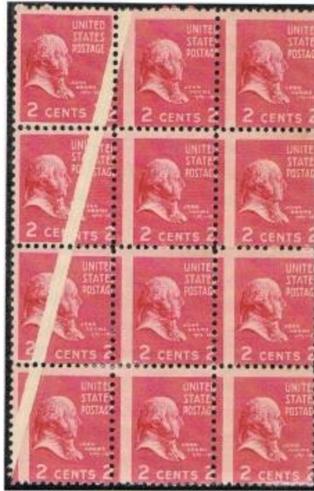
Figure 9. Mis-spacing of vertical perforations due to a pre-printing paper crease that was opened before perforating.
